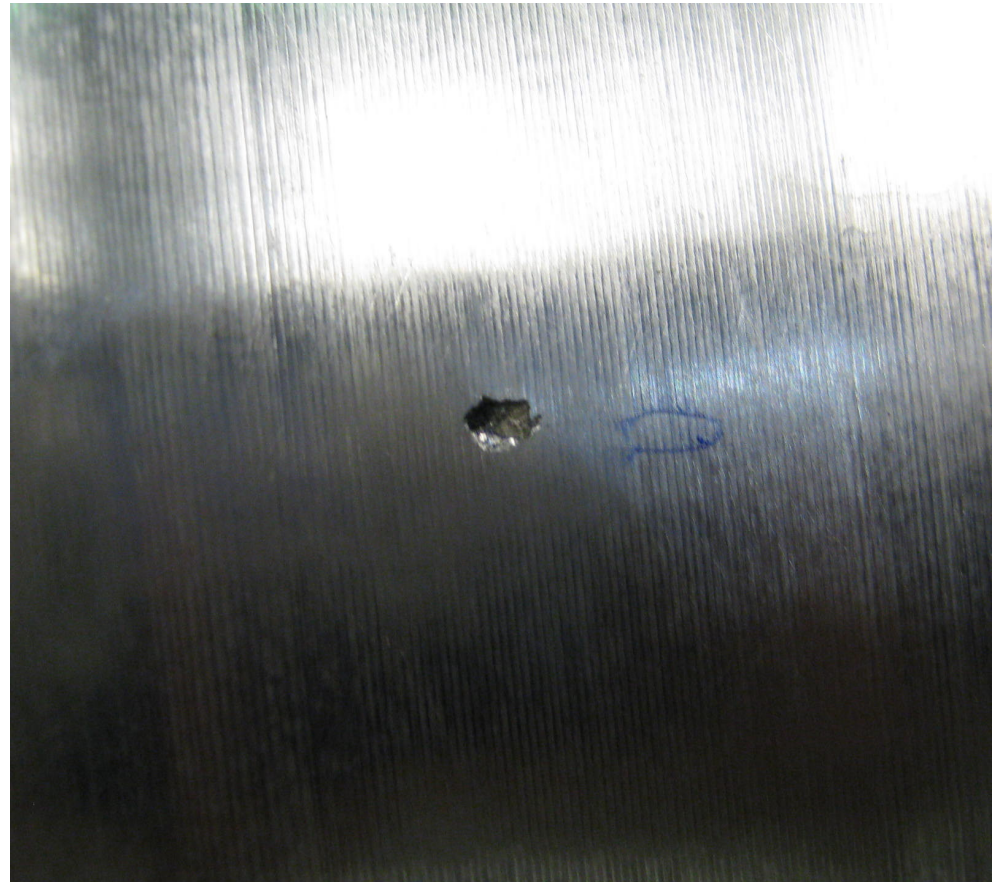
PIT IN BARREL LARGER THAN 6MM
