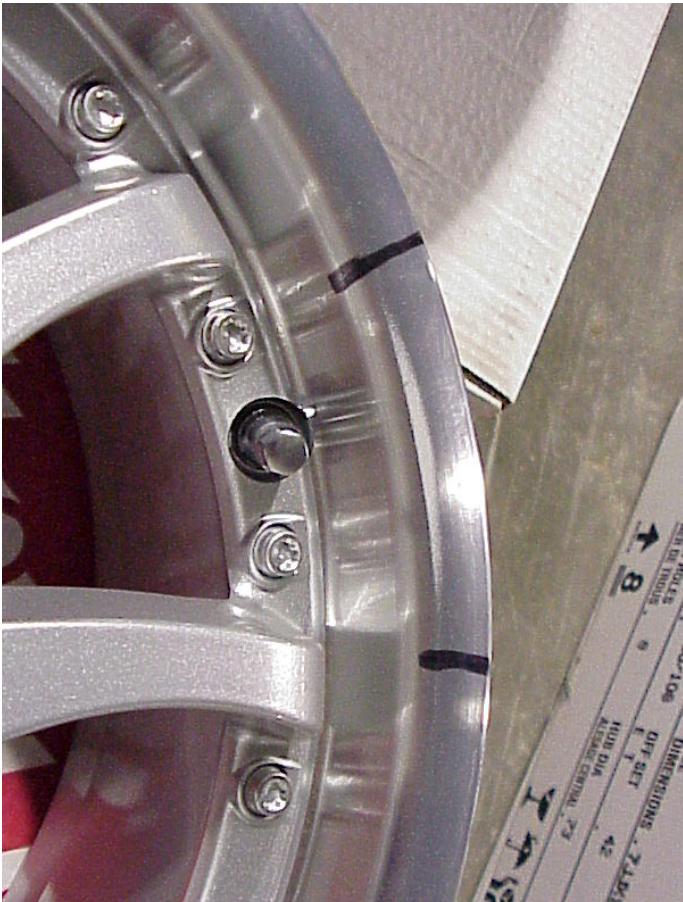
MISSED PAINT ON THE MACHINED LIP
